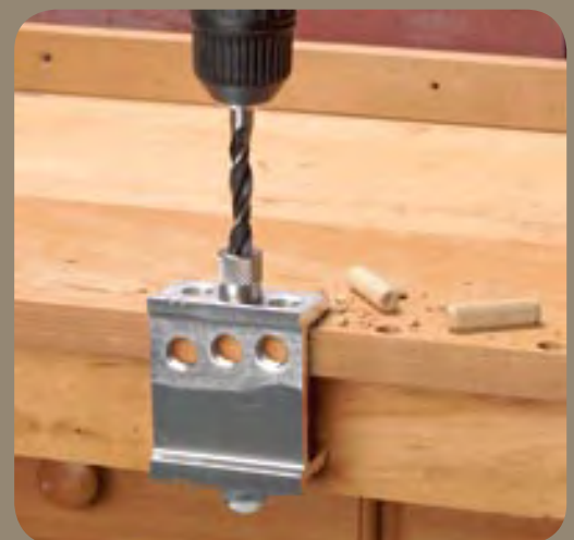
ABOVE: A simple dowelling jig
